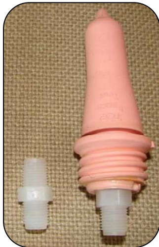
Figure 14. Peach Teat™ with a check valve to overcome leakage caused by high head pressure in a milk tank. The check valve in the photo has stainless steel and plastic components that resist the effects of acidified milk.
