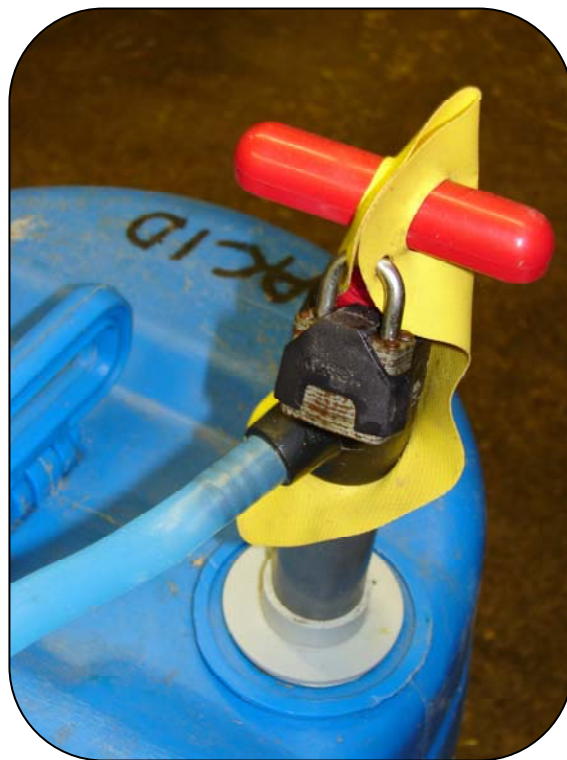
Figure 19. A padlock used with the yellow strap-lock prevents unauthorized dispensing of formic acid.
