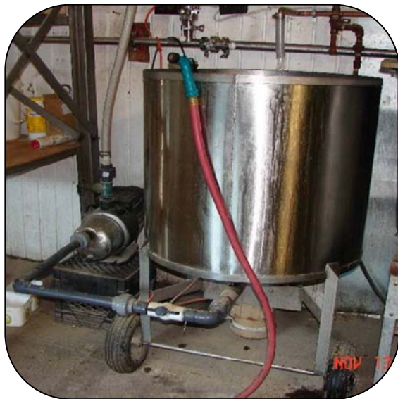
Figure 3. Batch mixers save time and improve the quality of mixtures. This 300 L mixer has a bottom-mount motor that spins an impeller. It easily handles the 133-166 L needed to mix a 20-25 kg bag of powder. A pump transfers the milk to a bulk milk tank. Brian St. Denis is the Ontario distributor – 450-451-0078.
