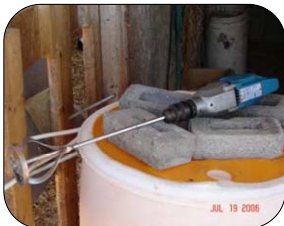
Figure 16. An electric drill and a paint stirrer attachment do a very good job of mixing. Several producers made mixers to insert into their electric drills. It is essential to select a mixer for the size of the container and volume of milk.
