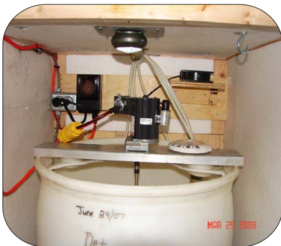
Figure 9. The interior of the warm box provides spacious accommodation for a 200L barrel, nipple bar, agitator, timer, heater, fan, light and thermometer.
